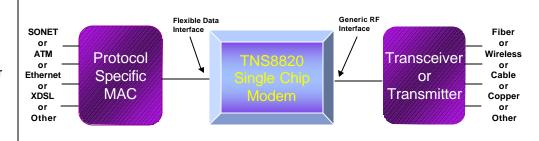
Power Consumption: approximately 4 Watts Package: 352 pin BGA
